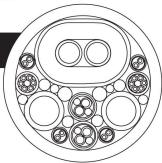
Our customers are always moving toward more compact medical devices with greater functionality. Our ability to extrude extremely fine walls of Teflon coupled with our ability to integrate air lines into our medical cables provides our customers the means to reduce size drastically.
